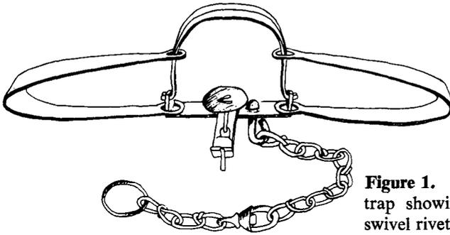
**Figure 1.** Modified No. 11 Victor trap showing the location of the swivel rivet and chain swivel.
